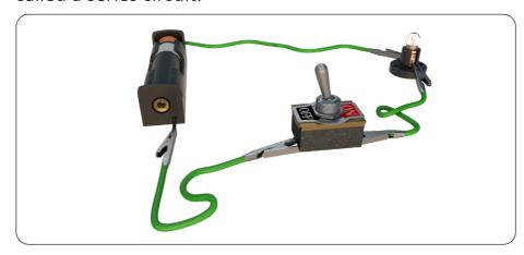
When electricity flows through all the components of a circuit, it is called a complete circuit.
