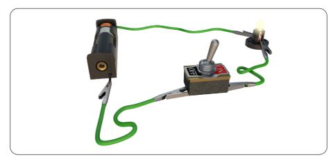
When electricity cannot flow through all the components of a circuit, it is called an incomplete circuit. Loose wires, damaged components and flat cells or batteries can all stop the flow of electricity around a circuit.
